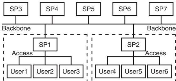
The introduction of Ethernet and/or ATM into the “last mile” infrastructure, over DSL or cable media, make an access network capable, in theory, of providing switching and/or routing capabilities, facilitating equal access scenarios.
