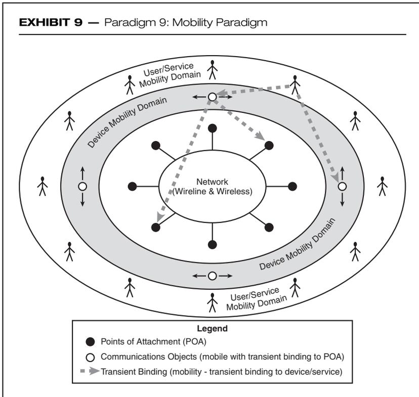
seen from Exhibit 9 that there is no permanent relationship between the identity of an object (e.g., user or device) to be involved in a communication and its location (i.e., the place in which it can be found). In all cases, a transient relationship is established between the communication object and a location. Thus, in general terms, the location/place of a given object can be represented by the physical point of attachment (POA), at which the said object can be reached/found.
