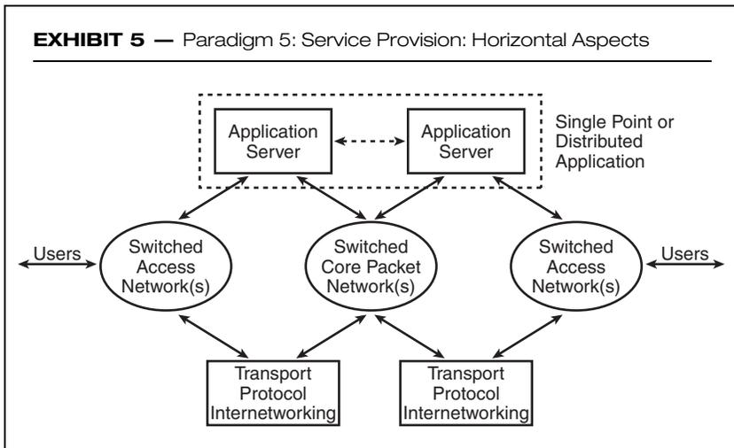
an access network needs to be made. The network segment used to access a server
