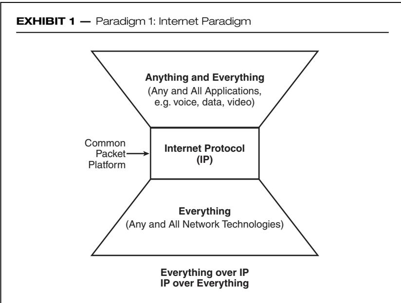
telecommunications technologies.<sup>2</sup> Because IP functionality is the only functionality “seen” by the layer(s) above IP, any particular functionality offered by the underlying telecommunications technology is (largely) ignored and not used.
